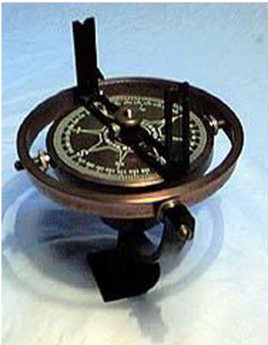
An example of a pelorus. Its graduated disc is mounted on gimbals and can be rotated and clamped so as to “repeat” the compass dial. An outer ring has opposite marks for alignment with the fore and aft axis of the ship. The sighting vanes can also be rotated and clamped on required bearings.
